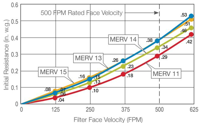
Maximum recommended final resistance for all VariCel® VXL filters is 2 in. w.g.\*
